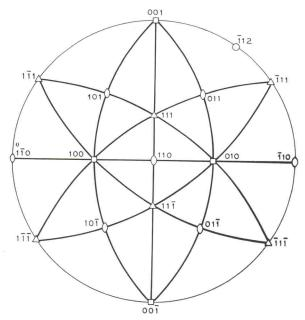
Fig. 2. Standard (110) stereographic projection for a cubic crystal.
